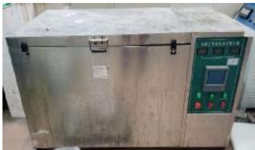
Figure 2. Concrete freezing-thawing test box
