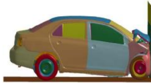
Figure 2. The finite element model of car frontal crash
