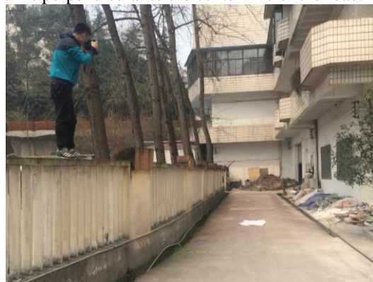
Figure 1. Close-range Photogrammetry of the Road
