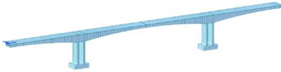
Figure 2. FEM of the full-bridge(Midas Civil)
