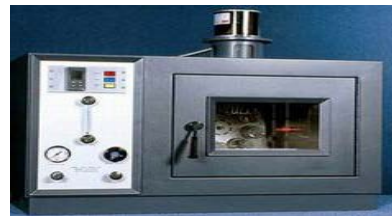
Figure 2. The thin film oven aging test (TFOT)
