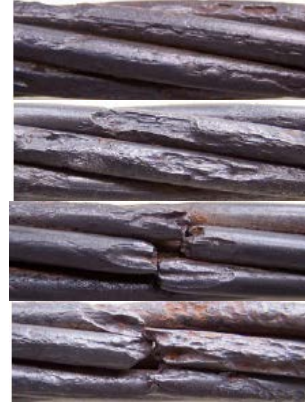
Figure 2. Static Tensile Test (Corrosion result)
