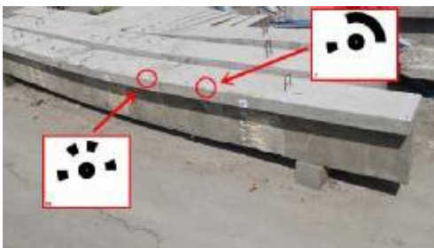
Figure 3. Layout of mark points in the middle of T-beam
