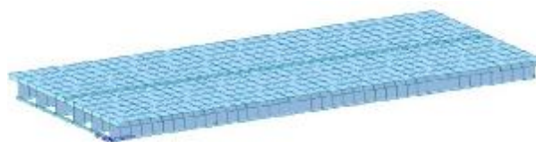
Figure 18. The finite element model of long-term bridge
