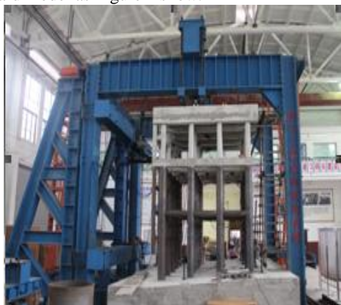
Figure 2. Structural static / dynamic test system
