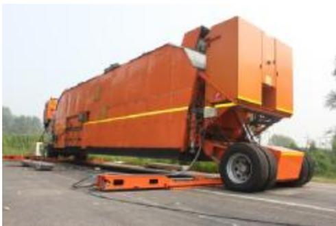
Figure 2. Curve: MLS66 accelerated loading equipment
