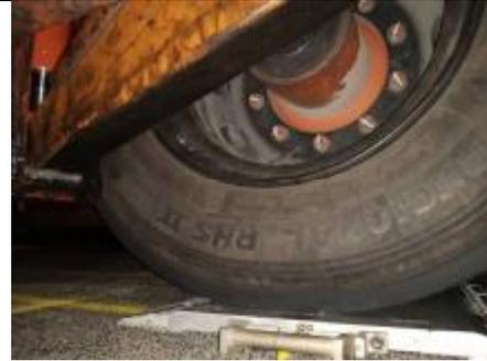
Figure 3. Curve: MLS66 half-axis double-wheel loading unit
