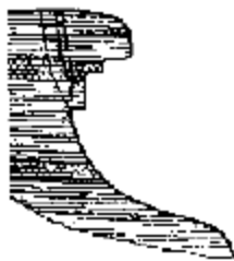
Figure 1. Fall type dangerous rock 图 1. 坠落式危岩
