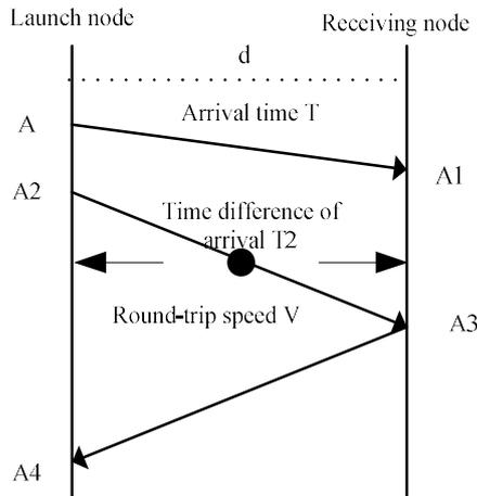
Figure 6. Self localization data transmission process of mobile node
