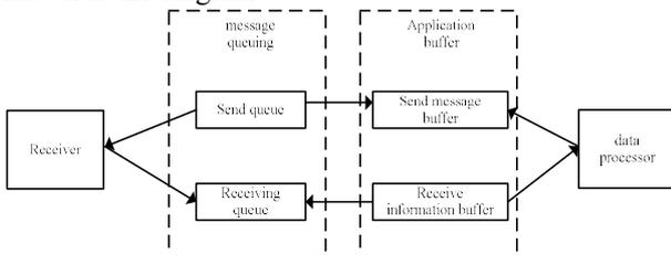
**Figure 8. Single port pipelining information transmission mechanism**
