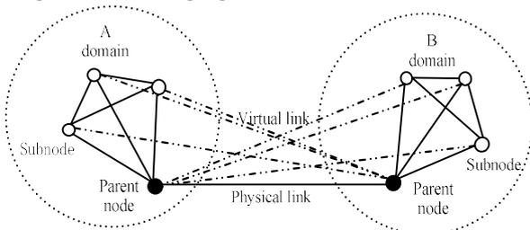
Figure 2. Distributed virtual network optimization structure
