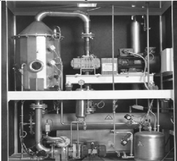
Figure 3. MVR heat pump falling film and evaporation experimental platform
