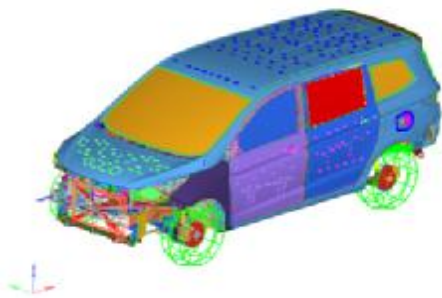
Figure 4. The Finite Element Model of the Full Vehicle 图 4. 整车有限元模型
