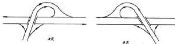
Figure 2. Trumpet Interchange. 图 2. 喇叭形互通立交
