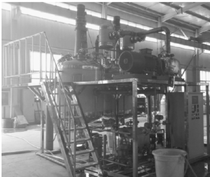
Figure 2. Jacketed MVR heat pump concentrating and evaporating system
